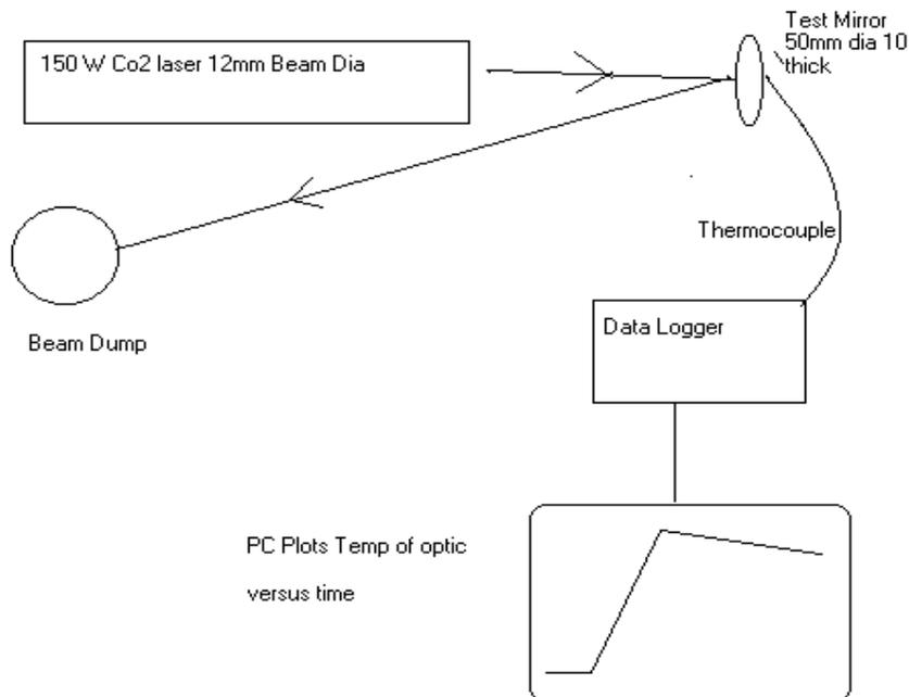
The rate of heating of the mirror is measured by a precision thermocouple attached to the mirror. Knowing the heat capacity and mass of the mirror allows the rate of heating to be converted to the amount of the beam absorbed. Traditionally absorption is expressed as a percentage, but units of parts per thousand can give a better idea of scale, 0.1% = 1 part per thousand, 0.5% = 5 parts per thousand, etc.
