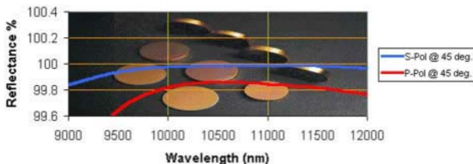
**Phase retarders** – A vacuum deposited dielectric coating that introduces a  $\frac{1}{4}$  wave phase shift. This circularly polarizes a linearly polarized beam. Very sensitive to incident angle (45 degrees) and wavelength (10.6 microns). Can be made on copper or silicon.
