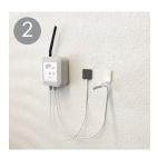
2. Place the sensor nodes on the inner wall, ensuring they are no more than 100m from the base station. Check connection to the base station.
