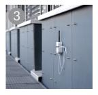
3. Place sensor node for the outer temperature measurement at about the same height as the inner sensor node inside the building. Measurement process starts automatically with start of the base station.
