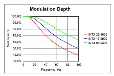
The "slowest" Intex part INTX 22-1000 can be chopped at up to 70 Hz before the modulation depth goes below 50%. The fastest, INTX 08-0300 can be electronically chopped up to 140 Hz. with modulation above 60%.
