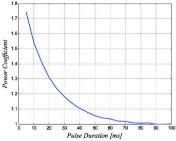
For voltage pulses where t < 50 ms, you can adjust the voltage and power experimentally. For this, you must use a fast-response (0.5 ms or less) detector to measure the emitter temperature. Perform the initial calibration of your detector with nominal-voltage pulses. The measured amplitude of the output signal corresponds to a
