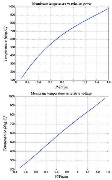
For short pulses and duty cycle 50% you can evaluate power coefficient from the graph and correct power.
