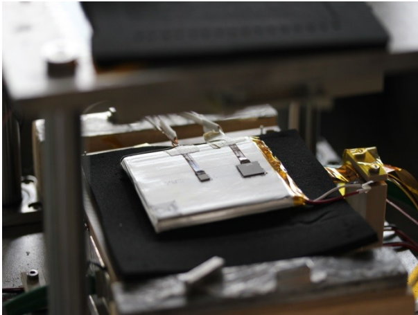
Figure 2: Calorimetric footprint of a Li-ion pouch cell (Renata) during battery cycling at isothermal conditions recorded with two different heat flux sensors from greenTEG (gSKIN-XP and gSKIN-XM); left: measurement setup; right: measurement results
