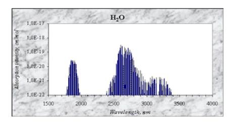
Water has very strong absorption band at 2550-2750 nm and 1830-1900 nm. When applying IBSG LEDs and PDs it is more preferable to use the second absorption band at 1830-1900 nm since emitters and detectors for this spectral range provide much better efficiency (the data are taken from HITRAN Catalog).
