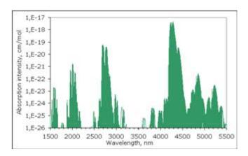
Carbon Dioxide has very strong absorption band at 4200-4320 nm. Other not so strong absorption bands that can be used for detection are located around 2700 nm and 2000 nm. (The data are taken from HITRAN Catalog).
