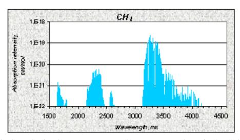
Methane has the main absorption band at 3200-3400 nm. Other not so strong absorption bands that can be used for detection are located around 2300 nm and 1650 nm (the data are taken from HITRAN Catalog).
