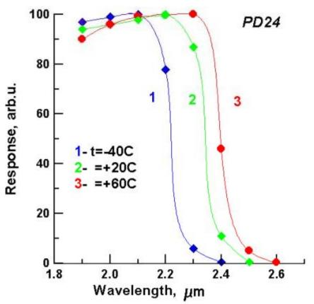
Long-wavelength edge of the spectra, measured at different temperatures and temperature dependence of the dark current for PD24-02 is presented here. Temperature dependences of the other models have the same shape.
