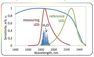
The spectra of an LED and a PD for H<sub>2</sub>O detection:
