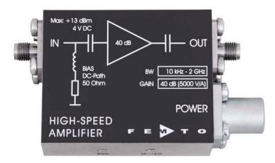
The well proven FEMTO GHz amplifier series HSA-X has been redesigned with bandwidths up to 2.5 GHz. For all HSA-X amplifier model the bandwidth has been extended. The 2 GHz models now have 2.2 GHz bandwidth at 40 dB gain and a 2.5 GHz bandwidth at 20 dB gain.
