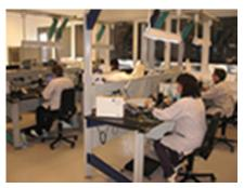
It has to be ensured both for visual inspections and for optical measuring methods that there are no disturbances due to external light. That is why eight production rooms and one measuring room were designed as dark spaces without windows and with black, non-reflective wall colour. These spaces range from  $3 \times 2$  square meters to  $23 \times 1.5$  square meters.
