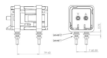
Drill hole 4 x Ø3 mm for level 2 mounting
