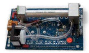
Infrared gas sensors: Chillcard NG Range SPECIAL CHILLCARD NG
