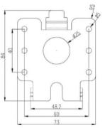
• Column type bracket can be installed on the Aisle gate
