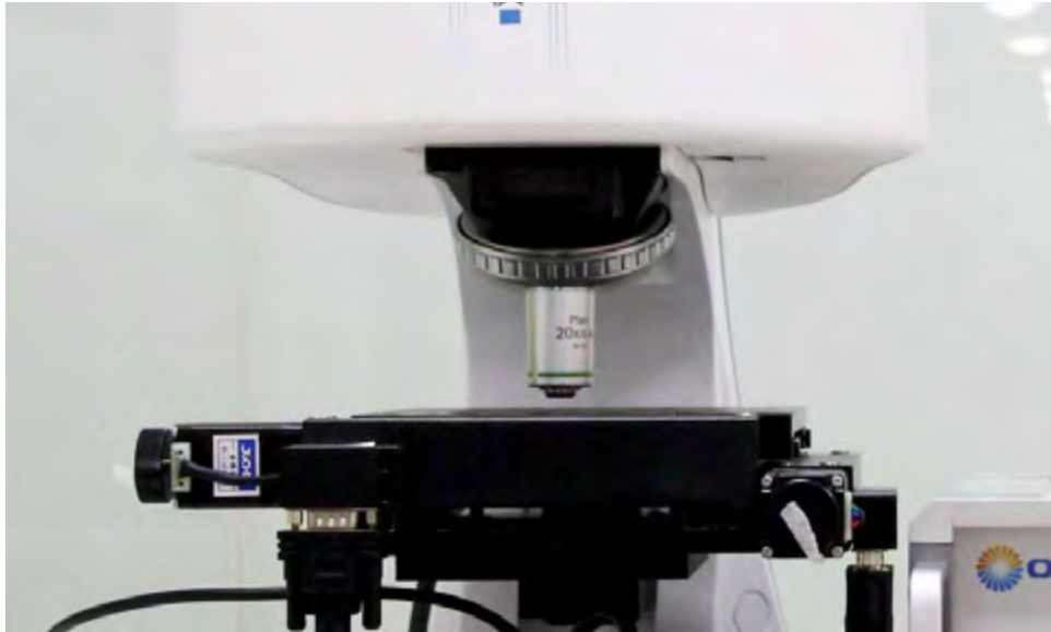
Fig 10 Raman signal high transmission objective, objective focal length up to 8mm
