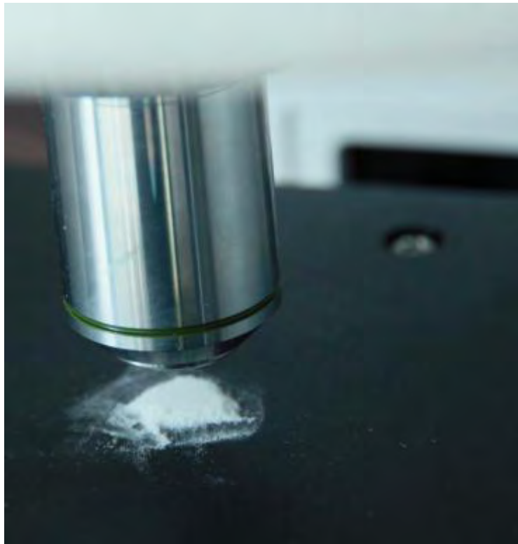
Fig 10 Raman signal high through put objective, objective as long as 8mm;
