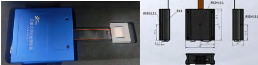
Fig.2. Physical and Dimensional structure diagram of FSLM-HD70-A/P (GW)
