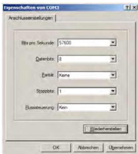
Figure 12: Setting up parameters in Microsoft Hyper Terminal
