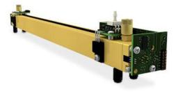
After the water is boiled the Silarex NDIR TOC sensor measures  $CO_2$  in the steam at 3 ranges – 0...100ppm, 0...1000ppm & 0...10,000ppm.  $CO_2$  is directly linked to the TOC concentration in the water. **Simple and precise!**
