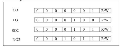
I<sup>2</sup>C Sensor Type Address: CO: 0x02 O3: 0x08 H2S: 0x06 SO2; 0x0A NH3: 0x10 NO: 0x1E NO2: 0x16 CH2O:0x22 PID; 0x42
