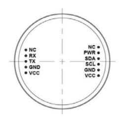
\* Note: Two VCCs are connected internally.
