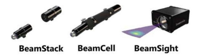
BeamCell uses a chamber like NDIR. BeamStack has the laser and detector modules separated across a path where you want to measure the gas concentration. BeamSight has the laser and detector in the same module and measures the reflected signal.
