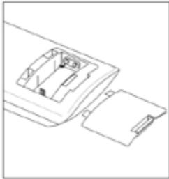
Open the battery cover in the back of main unit and check for a 9V battery is or isn't.
