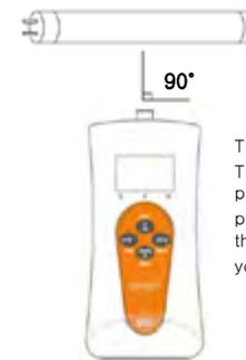
The sensor is located on the top of the body. The measurement surface of the sensor is positioned perpendicular to the UV light source or solar light that you want to measure.
