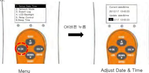
Move using the left and right buttons and press the UP and DOWN buttons to increase or decrease the number.
