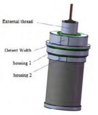
6.1 As shown in the figure above, when the product is installed with external thread, the wrench with 46mm opening on the opposite side should be used first to clamp the clamp, and then start the operation, while avoiding the force on other parts of the product;
