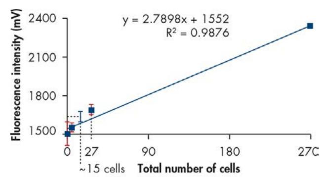
Efficient detection of viable cells. Error bars are shown in red. The blue error bar represents the extrapolated data of detectable cells. The total volume was 300  $\mu$ l and a total of 27 cells in 300  $\mu$ l were measured. A total of 15 cells in 300  $\mu$ l can be detected (extrapolated).
