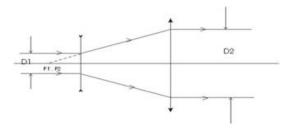
1) Parallel beam remains parallel after expanding with the beam expander; the amplification is D2/D1.
