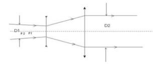
2) If the entrance beam is a converging beam, manual adjustment is required to reduce the distance between two lenses in order to make exit beam parallel.
